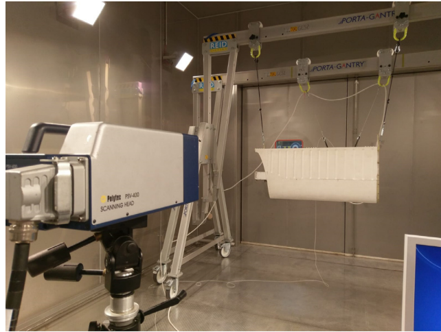
(a) test-rig and scanning laser vibrometer
