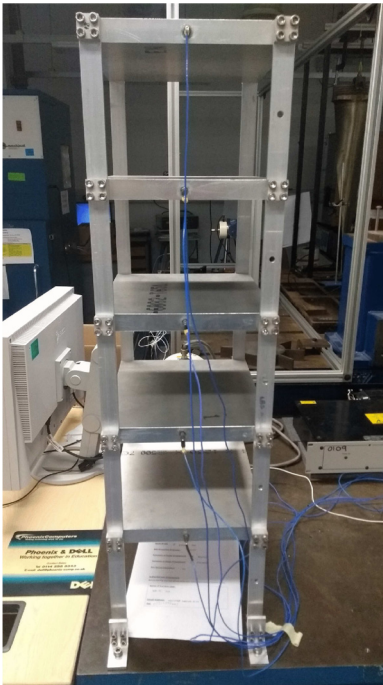
Fig. 8 Test setup of the representative five story building structure
