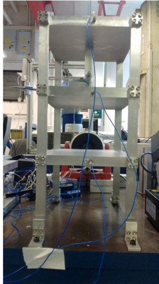
Fig. 9. Experimental setup of the three-storey building structure.
