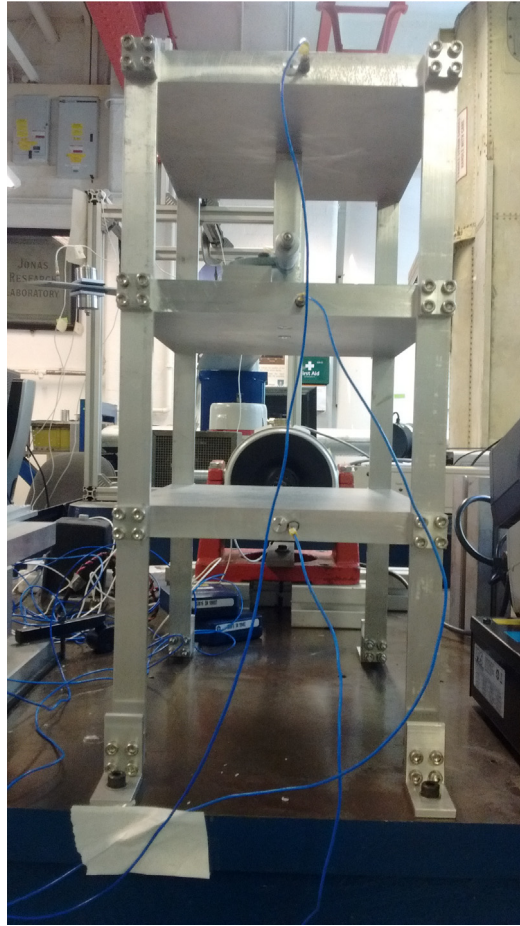
Fig. 24. Target domain structure: Experimental setup of three-storey building structure [4].
