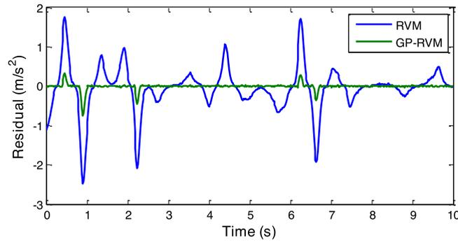
Fig. 6. Residual between the predictive mean and simulated response for RVM and GP-RVM method, first scenario (blue line: RVM method; green line: GP-RVM method).
