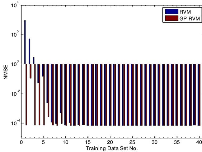
Fig. 10. NMSEs of the mean model prediction from the RVM and GP-RVM methods for the Silverbox test dataset (blue bar: RVM method; magenta bar: GP-RVM method).
