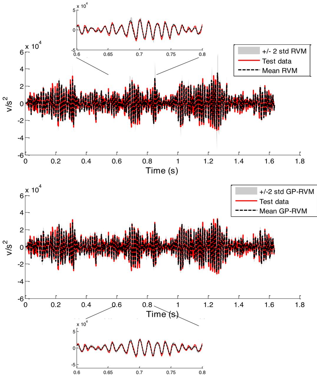
**Fig. 11.** Comparison of the Silverbox test data and model predictions from the RVM and GP-RVM methods (red solid line: simulated value; black dashed line: predicted mean of applied method; grey area: +/- 2 standard deviation of applied method).
