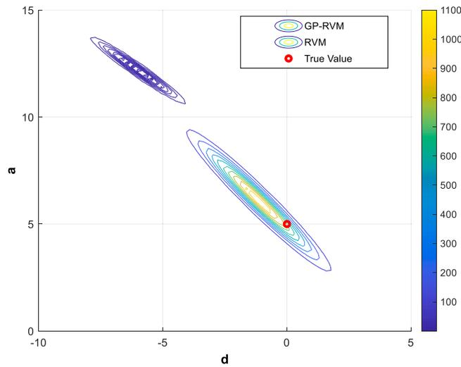
Fig. 4. Marginal likelihood against system parameters (red dot: true value; coloured contour: GP-RVM method; blue contour: RVM method).
